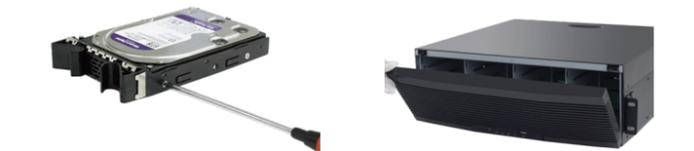
Use screws to fix the hard disk on the ejector lever. You can distinguish between the left side and right side in accordance with the indicators on the ejector lever.
